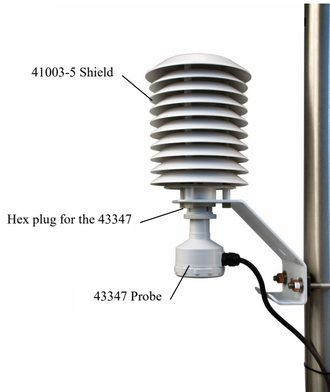
FIGURE 7-7. 41003-5 Radiation Shield mounted to tripod mast
