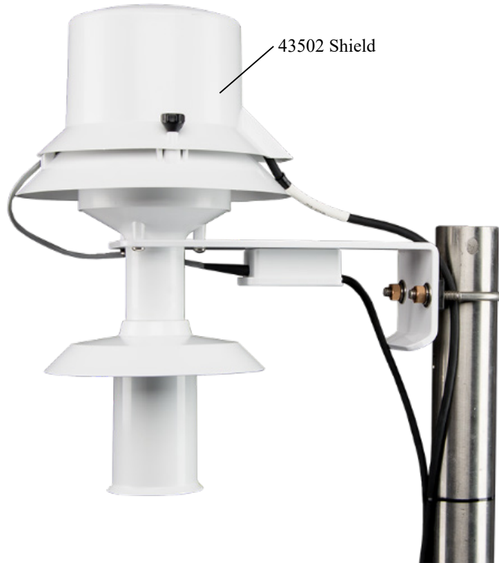
FIGURE 7-1. 43502 Radiation Shield mounted to tripod mast
